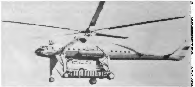
Figure 6-57. Mi-10 HARKE. A Soviet version of the flying crane concept is the HARKE, which also appears in a sling model. The HARKE is shown here in civilian markings.
